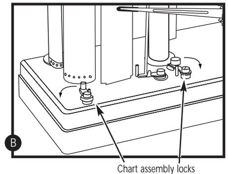
4. Pull the chart assembly back using the handle located behind the chart assembly. To prevent the unit from tipping over, hold the base of the instrument with your other hand. Use the handle to keep the chart assembly in a horizontal position.
