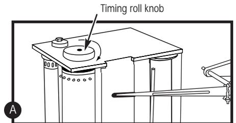
2. Wind the old chart paper onto the *Take-Up Roll* by turning the *Timing Roll* knob clockwise (in the direction of the arrow).
