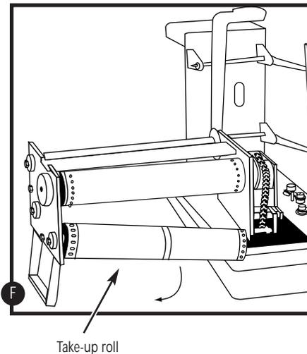
7. Replace the *Take-Up Roll* with the empty cardboard tube into the chart assembly.
