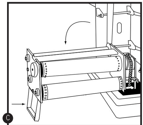
5. Remove the empty cardboard tube from the *Chart Roll* (see sticker on top of chart assembly for position).
