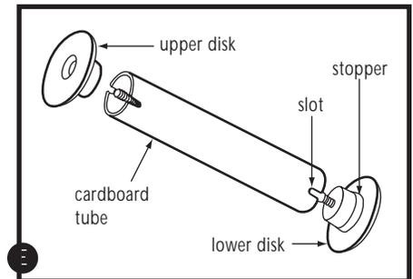
9. Install the *Chart Roll* with the new chart paper back into the chart assembly.
